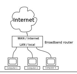
You should connect a straight TP network cable between the network socket in your apartment and the "WAN" or "Internet port" on the broadband router. Your computers should then be connected to the "LAN" or "Local ports" on the broadband router.
